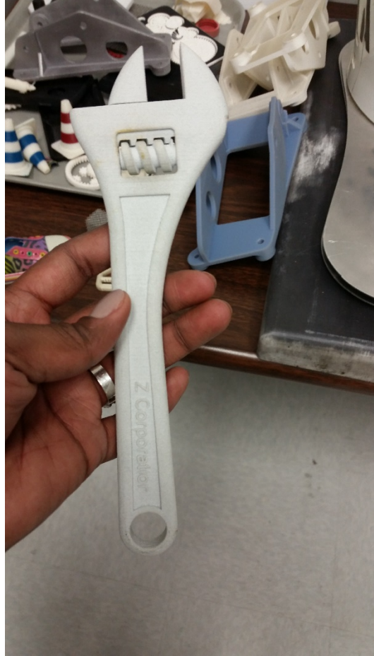
Wrench produced from binder jetting
