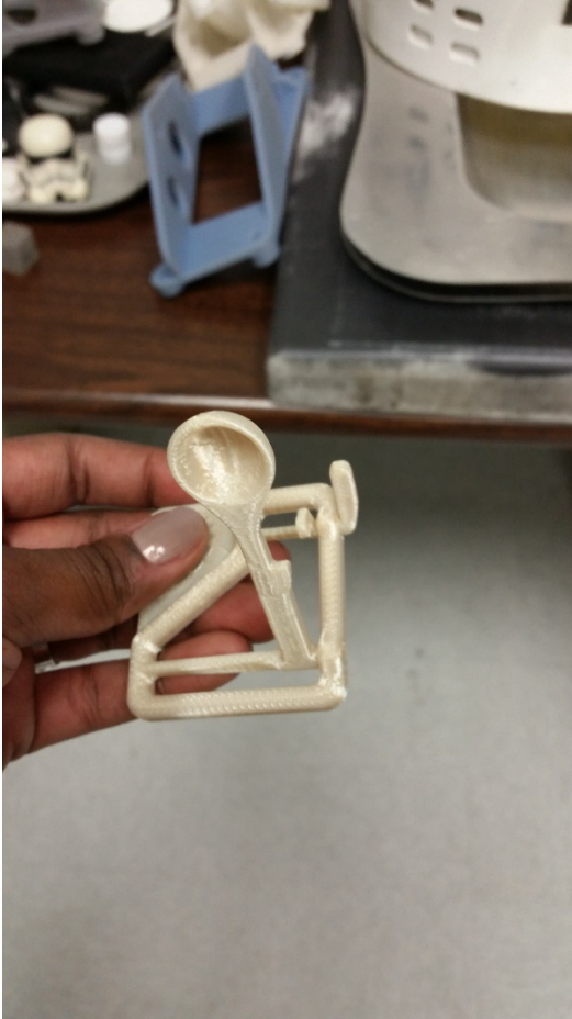
Mini catapult produced from FDM
